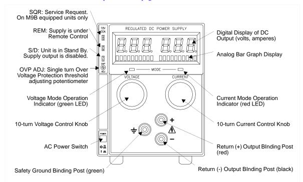
Figure 1.1 500 Watt Series Power Supply Front Panel
