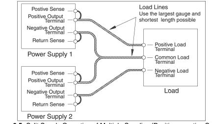
Figure 3.5 Split Supply Operation of Multiple Supplies (Positive-negative Supply)
