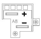
Figure 1.4 Output Busbars - note polarity markings (Low Voltage Models)
