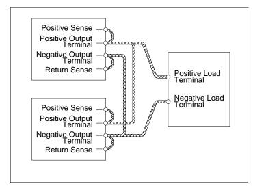
Figure 3.3 Parallel Operation
