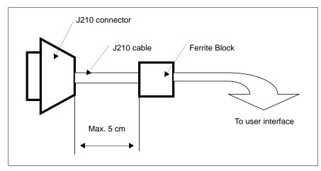
Figure 4.1 J210 User Cable with Ferrite Block
