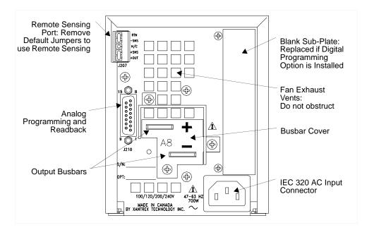
Figure 1.2 500 Watt Power Supply Rear Panel (7.5 V and 18 V)
