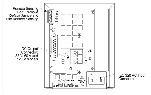
Figure 1.3 500 Watt Power Supply Rear Panel (33 V to 120 V)
