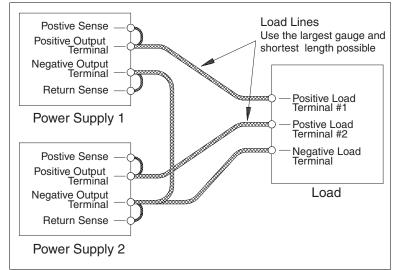
Figure 3.4 Split Supply Operation of Multiple Supplies (Two positive voltages)
