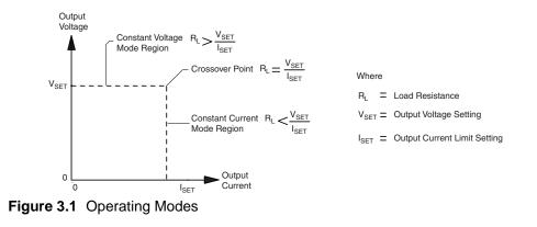
**Note** The control circuits have been designed to allow you to set output voltage and current up to 1.5% over the model-rated maximum values. The power supply will operate within these extended ranges, but we cannot guarantee full performance to specification.
